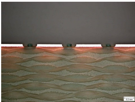
50 micron solder-dams (exposed using Olec ATH30)
